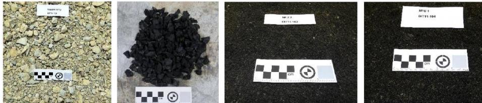
Figure 1. Subballast and rubber samples. (a) Unbound Granular Material-Subballast (b) Rubber 20 mm. (c) Rubber 2 mm. (d) Rubber 1 mm.
