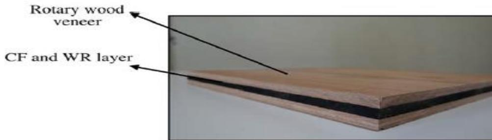
FIG. 2. Layers arrangement of the reinforced plywood panels.
