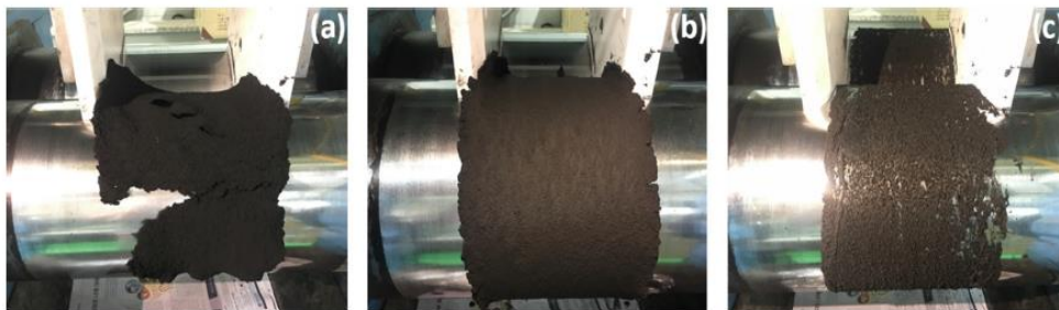
Different processing stages during reclamation of rubber, (a) stiff rubber hard to adhere to the roll, (b) moderate Mooney viscosity and easy to process, (c) sticky rubber easily adhere to tow rolls and also hard to process.
